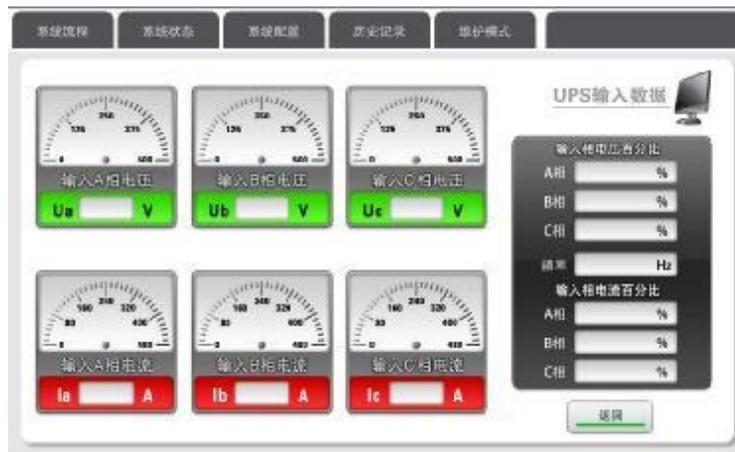
4. UPS battery and other data interface ( "System flow interface" click "Battery" or battery form to enter).
