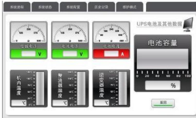
5. UPS output data interface (“system process interface” click “output” or output form to enter).
