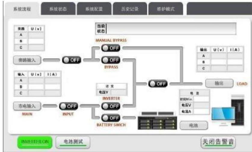
Click the inverter on button "INVERTER ON" or the inverter off button "INVERTER OFF", the password input window will pop up, enter the password "000000", click "ENTER" to confirm, turn on or off the inverter.
